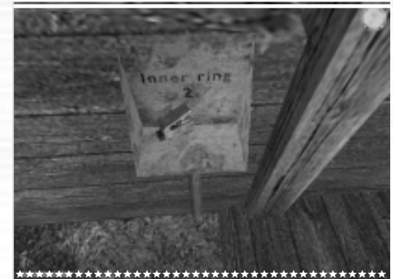
***** 19-4. These activators detonate explosives set along the perimeter fences. *****
